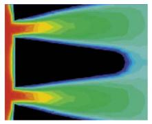
Fig. 3: Flow simulation showing the high flow velocities (red zone) at the wedge wire profile of the filter candle
